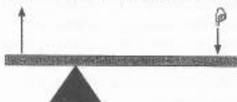
Figure 9.5 A diagram showing a first-class lever
