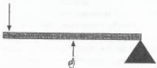
Figure 9.12 Diagram showing a third-class lever
